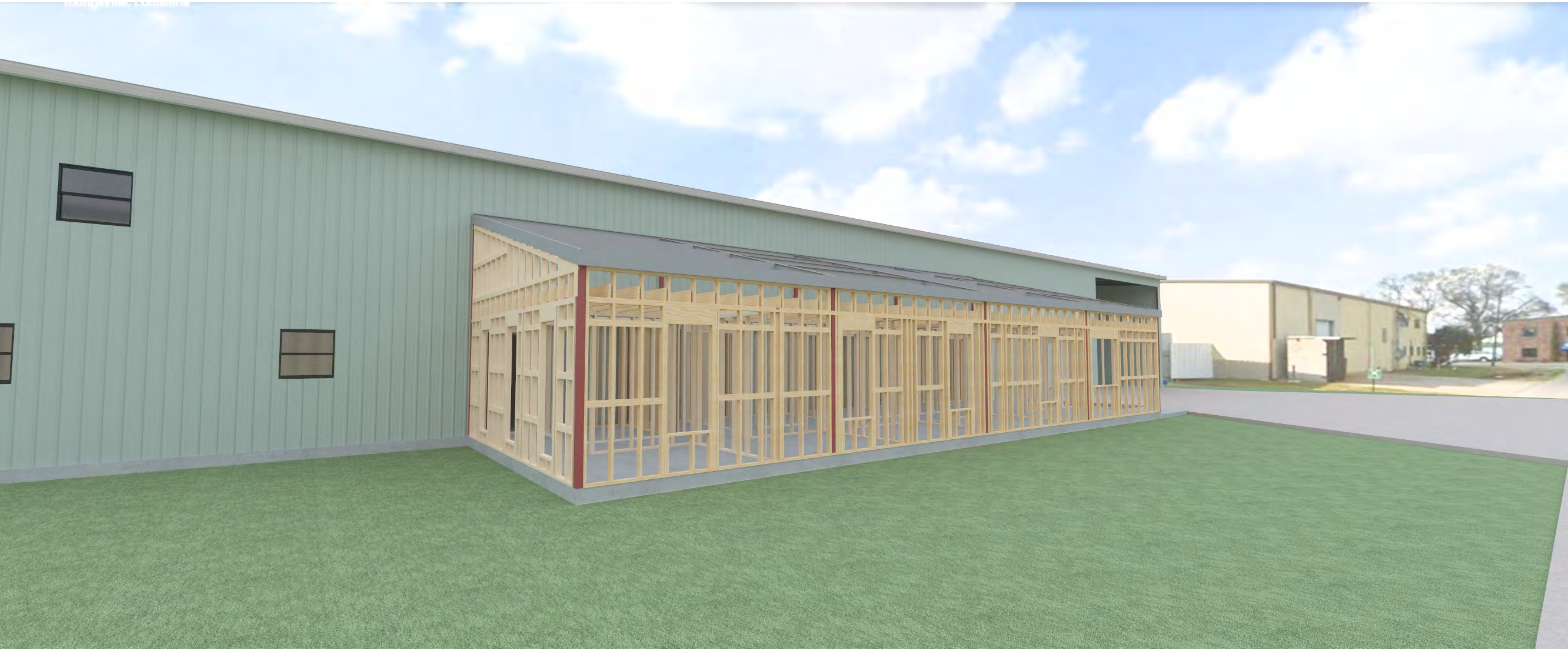
METAL ROOF SYSTEM WITH WOOD FRAMED WALLS & CEILING JOISTS
