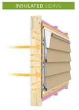
CedarMAX insulated siding performs an important function in a home's energy performance: breaking the "thermal bridge" between the home's studs and exterior cladding. Thermal bridging occurs when materials with poor insulating properties contact each other, allowing heat to flow through them.
