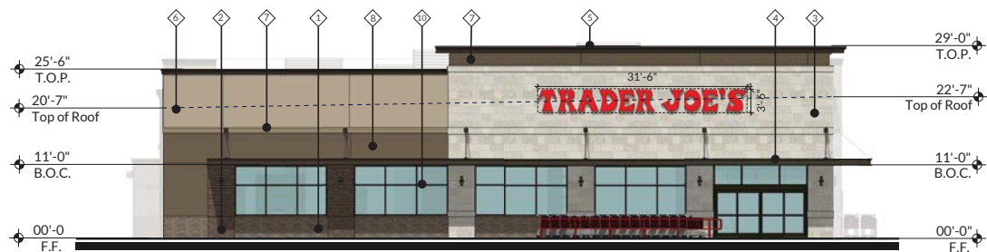
01 NORTH ELEVATION (FRONT) SCALE: 1/8" = 1'-0"
