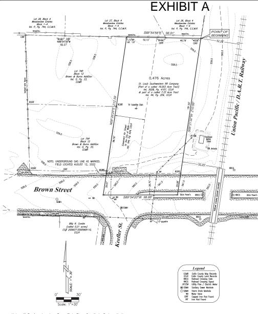
Notes: 1) Bearings based on Texas State Plane Coordinate System, North Central Zone 4202 (NAD83) 2) No part of the subject property is shown to lie within a Special Flood Hazard Area inundated by 100-year flood per Map No. 48085C0420J of the F.E.M.A. Flood Insurance Rate Maps for Collin County, Texas and Incorporated Areas, dated June 2, 2009 (Zone X); 3) This survey was performed with the benefit of Title Commitment GF No. LT—19135—1901352200021—BC issued February 23, 2022;
