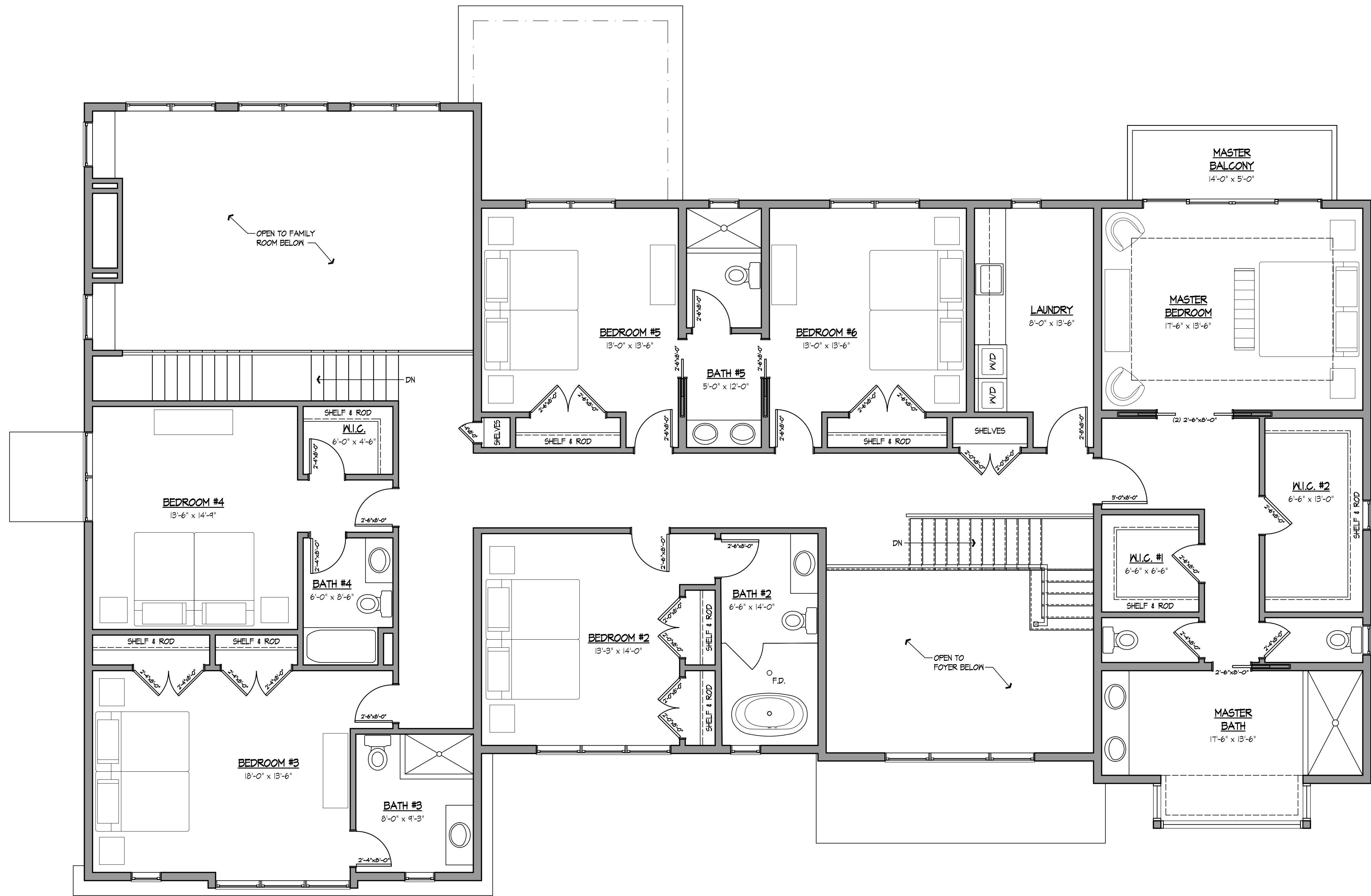
PROPOSED SECOND FLOOR PLAN SCALE: 1/4"=1'-0" FLOOR AREA = 2,880 SF
