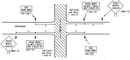
1. The typical minimum signing on a crossroad approach should be a "ROAD WORK AHEAD" (CW20-10) sign and a (G20-21) "END ROAD WORK" sign, unless noted otherwise in plans.
