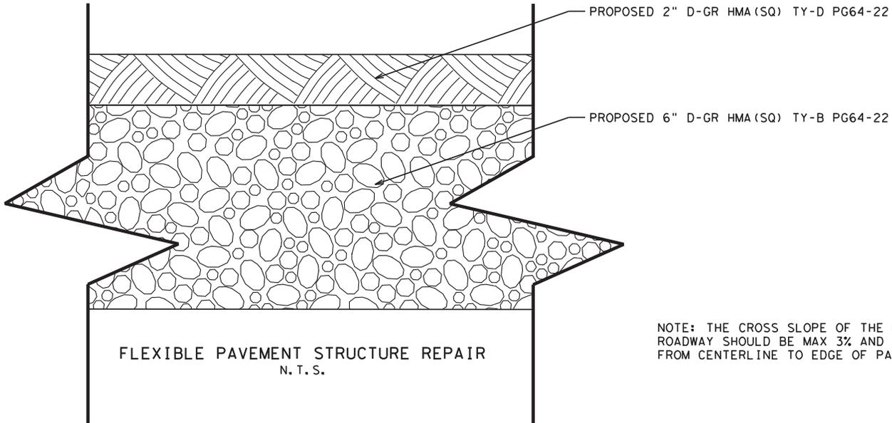
NOTE: THE CROSS SLOPE OF THE PROPOSED ROADWAY SHOULD BE MAX 3% AND A MIN OF 2% FROM CENTERLINE TO EDGE OF PAVEMENT
