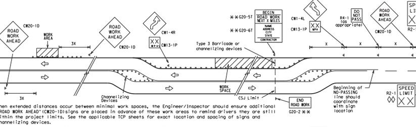
When extended distances occur between minimal work spaces, the Engineer/Inspector should ensure additional "ROAD WORK AHEAD" (CW20-10) signs are placed in advance of these work areas to remind drivers they are still within the project limits. See the applicable TOP sheets for exact location and spacing of signs and channelizing devices.
