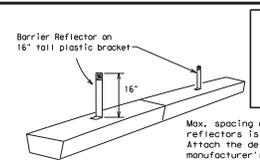
**LOW PROFILE CONCRETE BARRIER (LPCB) USED IN WORK ZONES**
