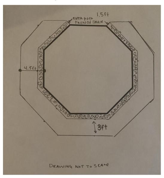
The final concept plan will involve an organic edged, natural rock border that roughly follows the pattern of the Gazebo. The plan includes a touch of site work to grade down away from the gazebo foundation for drainage with a small "French drain" style border around the base of the foundation. Plants would go in the outer bed rim in the fall (rainwater collection installation dependent) or in the spring of 2025.
