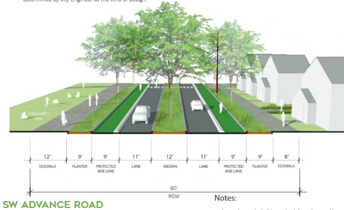
Figure 22. Cross Section of SW Advance Road
