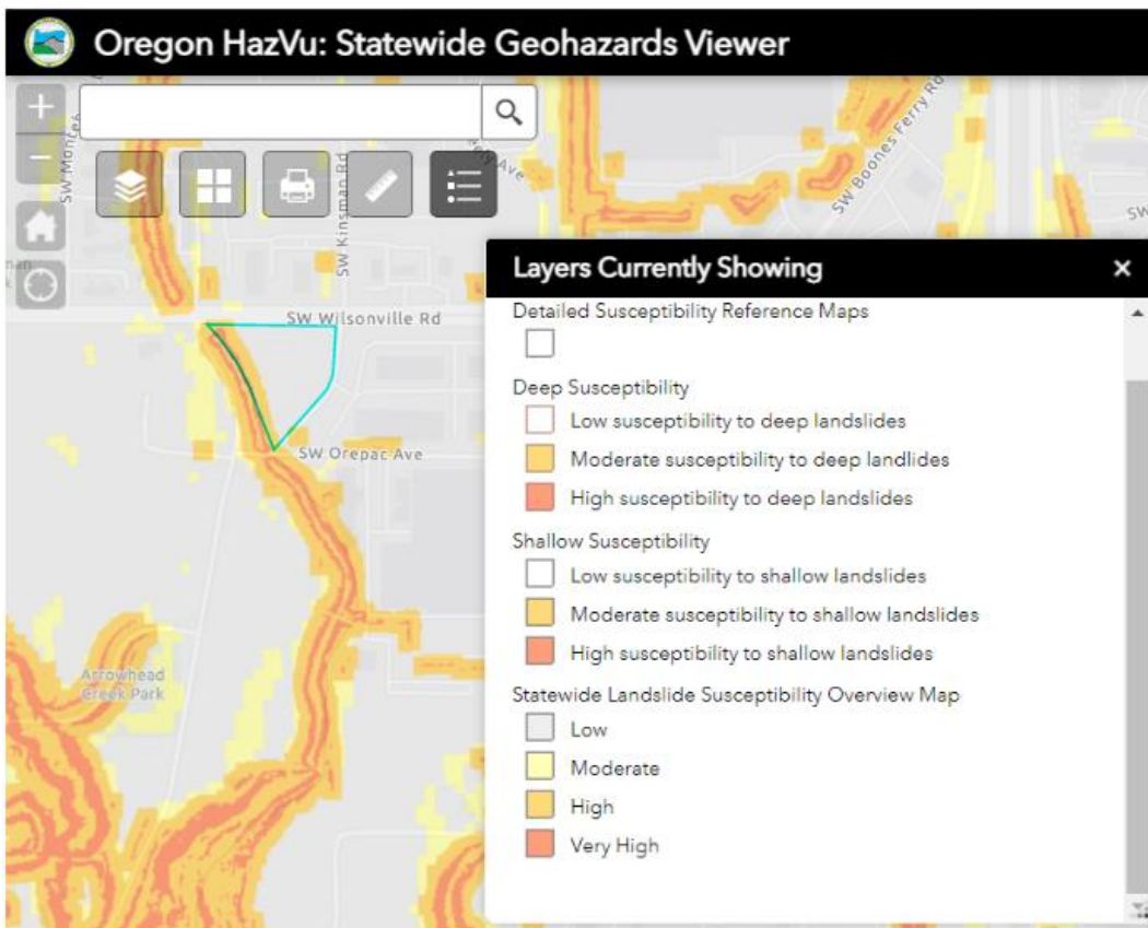
Figure III-1. Landslide Hazard Potential (DOGAMI)
