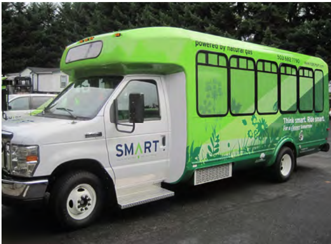
SMART Transit's 21-passenger compressed natural gas (CNG) buses offer a clean burning fuel alternative to traditional diesel buses.
