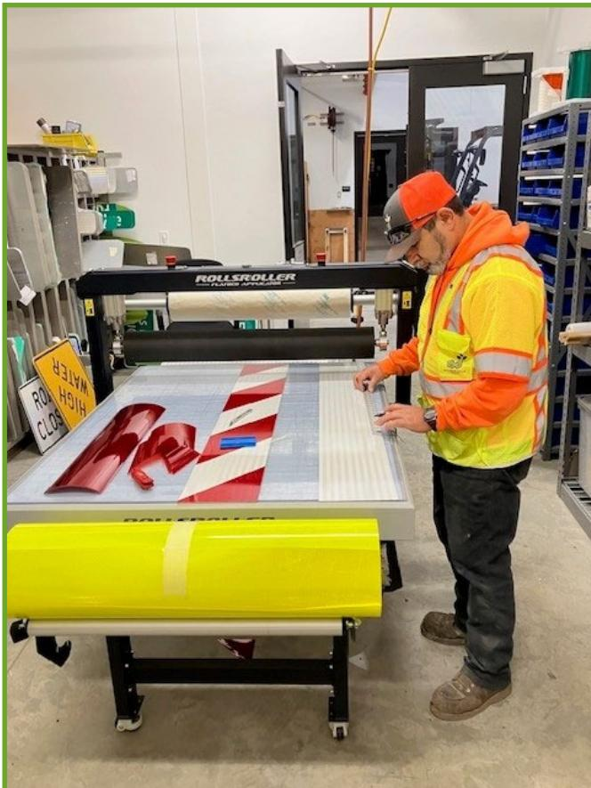
The Roads crew also made tidy work of replacing a few railroad crossing markings at the intersection of the rail tracks with Boeckman Road and Barber Street. Old pavement markings are ground off before new decals are applied and bonded to the roadway with heat.
