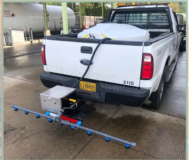
The City's new anti-ice unit, during final testing and adjustment.
