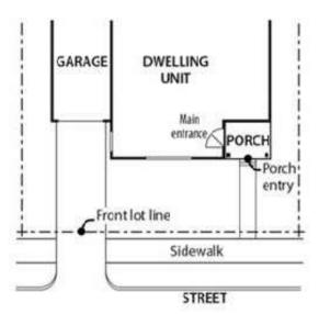
C. Distance from grade. Main entrances meeting the standards in subsection B., above, must be within four feet of grade. For the purposes of this Subsection, grade is the average grade measured along the foundation of the longest street-facing wall of the dwelling unit.
