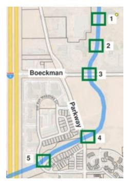
The project design includes modifications to the existing diversion structure and trapezoidal weir on the Siemens property north of Boeckman Road (1 and 2 in graphic), culvert replacement on Boeckman Road just south of the Siemens ponds (3 in graphic), and modifications to culverts that cross under Parkway Avenue and Ash Meadow Road (4 and 5 in graphic).
