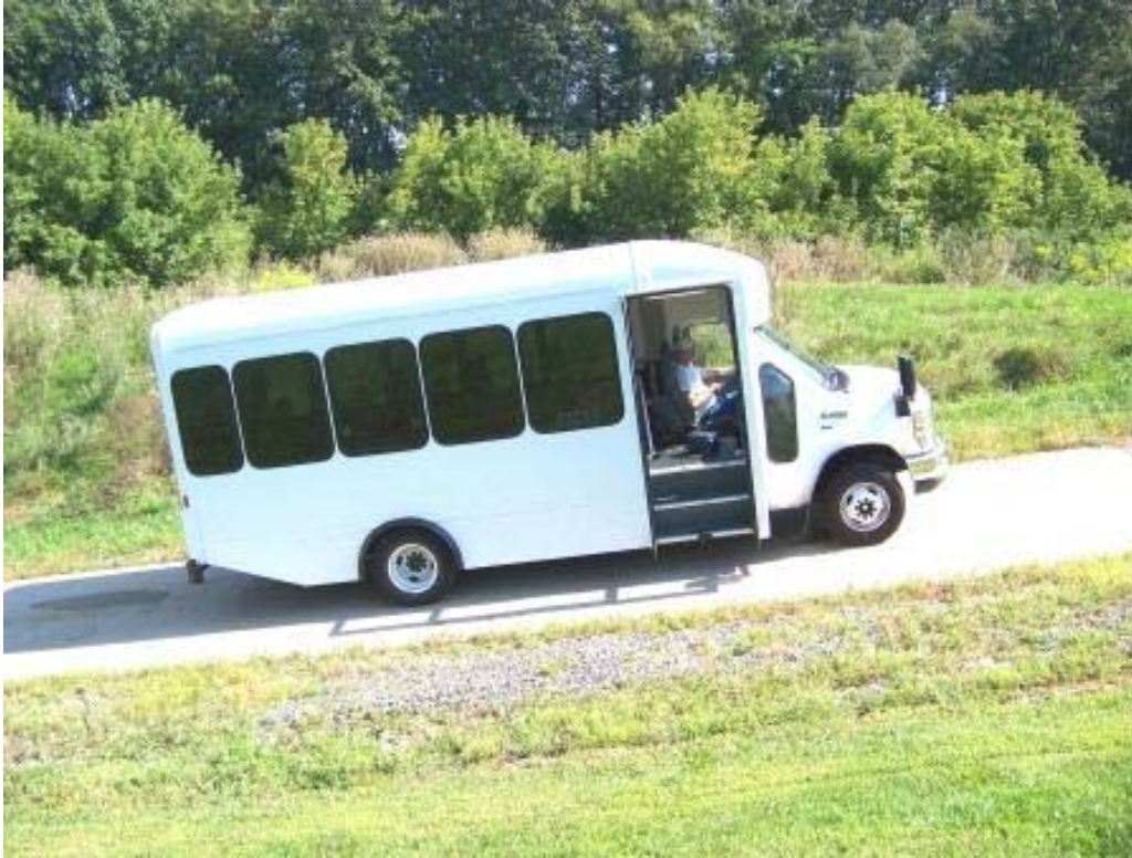
TEST BUS HELD UP AND DOWN ON 20% GRADE
