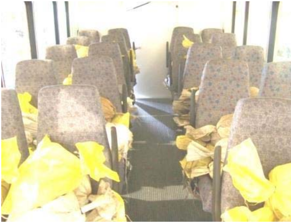
BUS LOADED TO 2.5 TIMES GVL (7,875 LBS)
