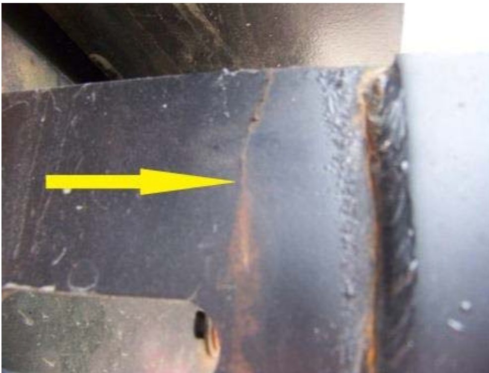
CRACKED LEFT AND RIGHT SIDE BUMPER BRACKETS (1,569 TEST MILES)
