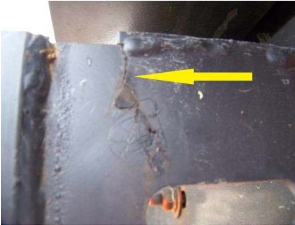
CRACKED LEFT AND RIGHT SIDE BUMPER BRACKETS (1,569 TEST MILES)
