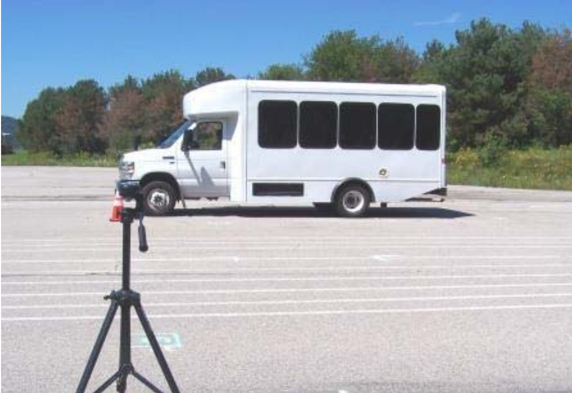
TEST BUS UNDERGOING EXTERIOR NOISE TESTING
