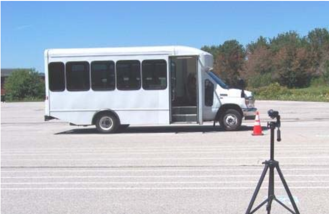
TEST BUS UNDERGOING EXTERIOR NOISE TESTING
