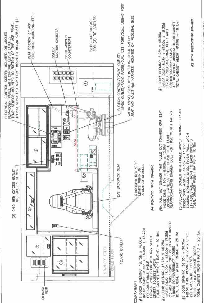
THIS DRAWING IS FOR REPRESENTATIONAL PURPOSES ONLY. DETAILS ARE CONCEPTUAL AND ARE SUBJECT TO CHANGE DURING DESIGN AND CONSTRUCTION DIMENSIONS ARE APPROXIMATE UNLESS NOTED OTHERWISE TO MEET A SPECIFIC CUSTOMER NEED.
