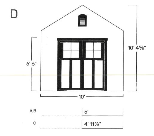
Measurements are to center from right siding edge
