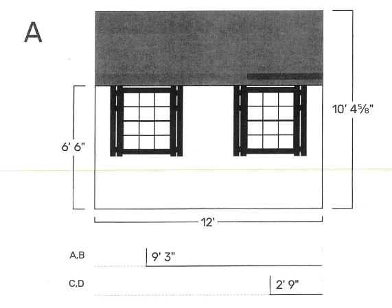
Measurements are to center from right siding edge
