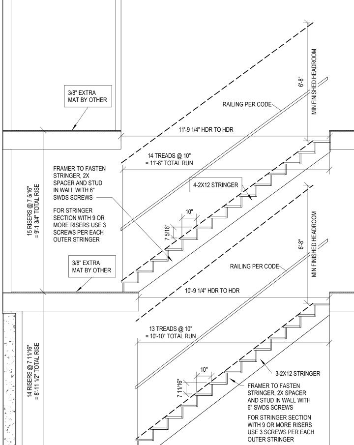
STAIRS ARE NOT TO BE INSTALLED UNTIL FLOOR IS POURED AND MUST BE FASTENED TO WALLS PER THE ABOVE NOTES
