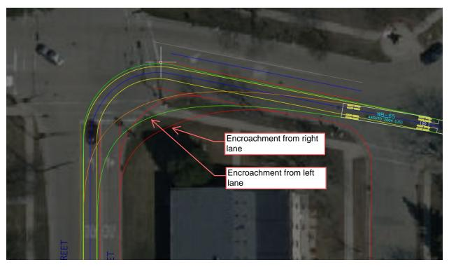
Turning Movement to Not Encroach on Grass/Sidewalk
