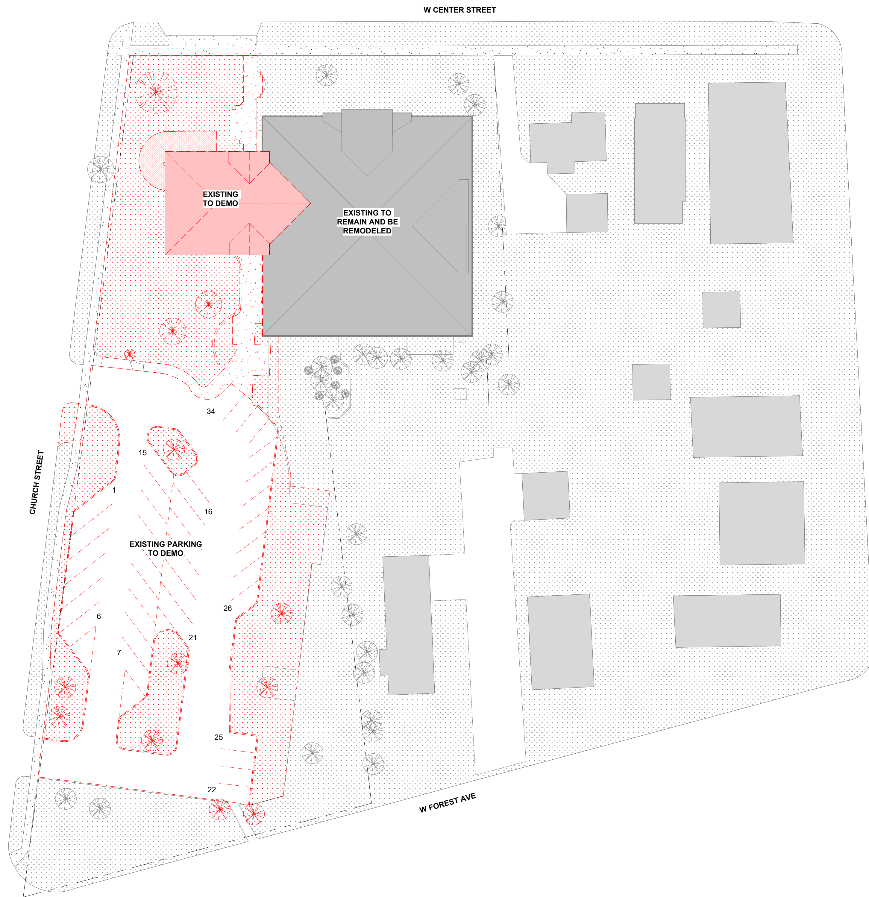
① Architectural Site Plan - Demolition 1" = 30'-0"
