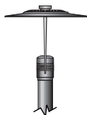
PHSC NEMA C136.41 7-PIN receptacle & shorting cap. Please consult factory to ensure electrical compliance.
