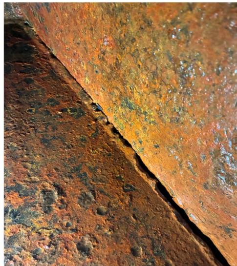
Figure 3 Failed Cell Wall and Underdrain Plate Weld Seam
