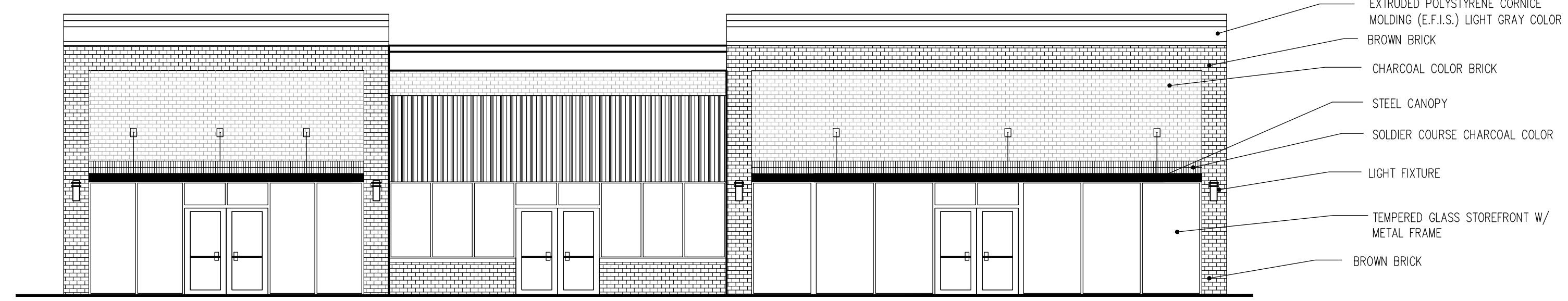
BUILDING "E" - PROP. FRONT ELEVATION SCALE: 1/8" = 1'-0"
