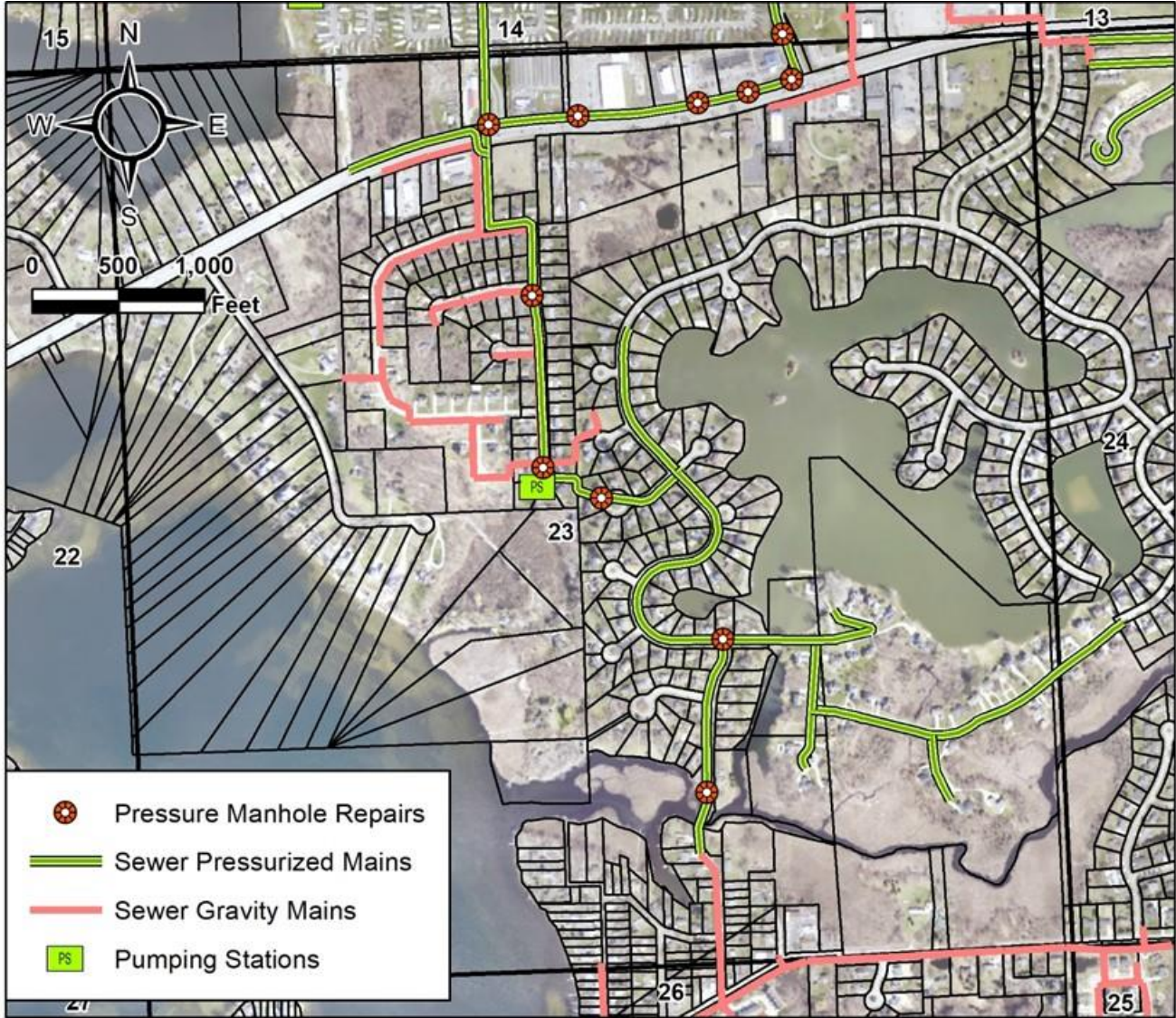
Figure 7 – Section 23 Repair Locations
