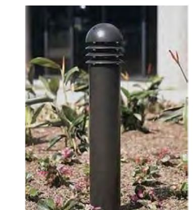
5M bollard light (4-CONDITIONS) BY LITHONIA LIGHTS OR EQUAL MODEL: DSXB LED (D-SERIES LED BOLLARD 8" DIA X 42" HGT.) OR EQUAL. ASYMMETRIC (12LED) 22 WATTS, 4000K
