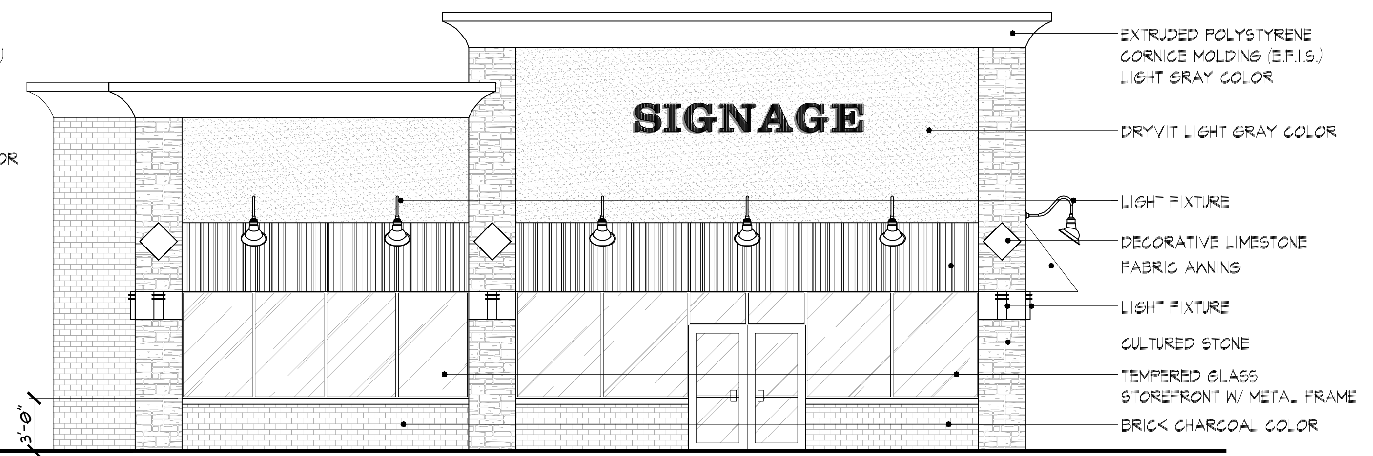
BUILDING "A" - PROP. FRONT ELEVATION SCALE: 3/16" = 1'-0"
