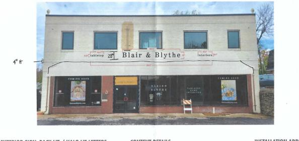
EXTERIOR SIGN, BACK LIT / HALO LIT LETTERS 1" Aluminum Letters Painted (Color TBD) Size: 392.5" x 20" Quantity: 1 Stud Mount to Building Face CONTENT DETAILS Overall content size: 392.5" x 20" Blair & Blythe: 185.5" x 20" Tabletop: 42.5" x 8.25" Interiors: 45.5" x 6.5" INSTALLATION ADDRESS 4812 rainbow Blvd , Westwood, KS 66205 Product Number: 1 Proof Number: 2 Additional proofs after #2 are S25 each
