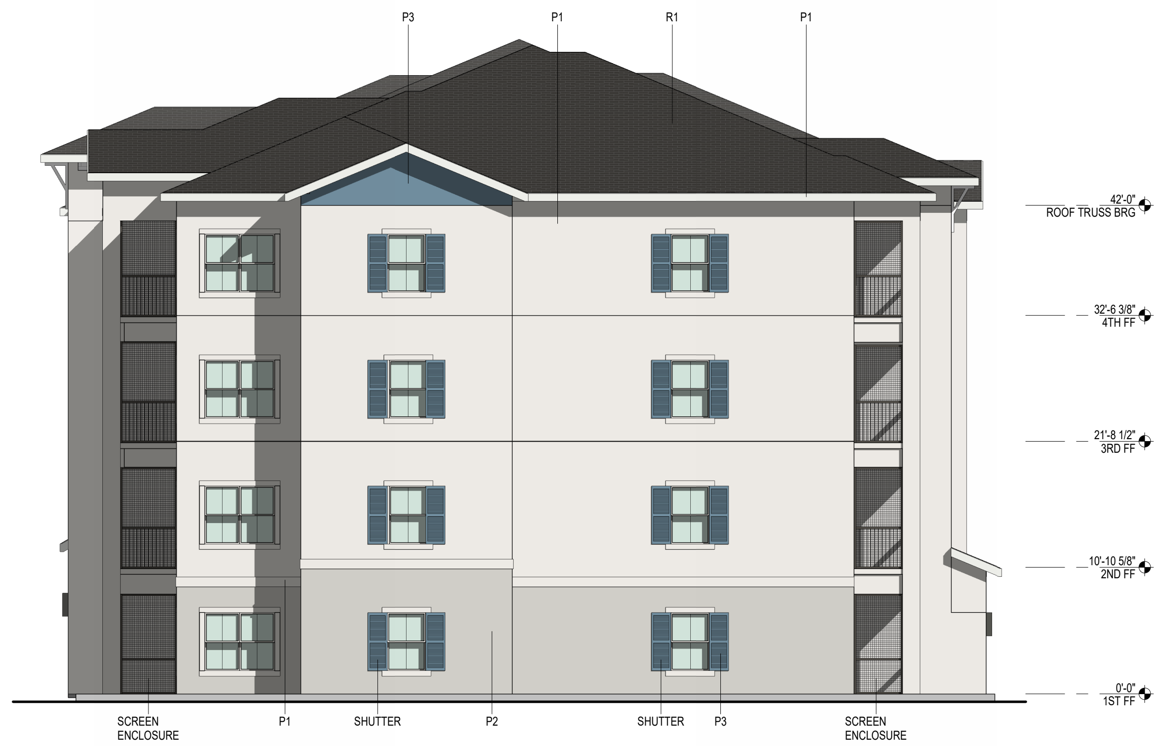
3 Building Type II - Left Side Elevation 1/8" = 1'-0"
