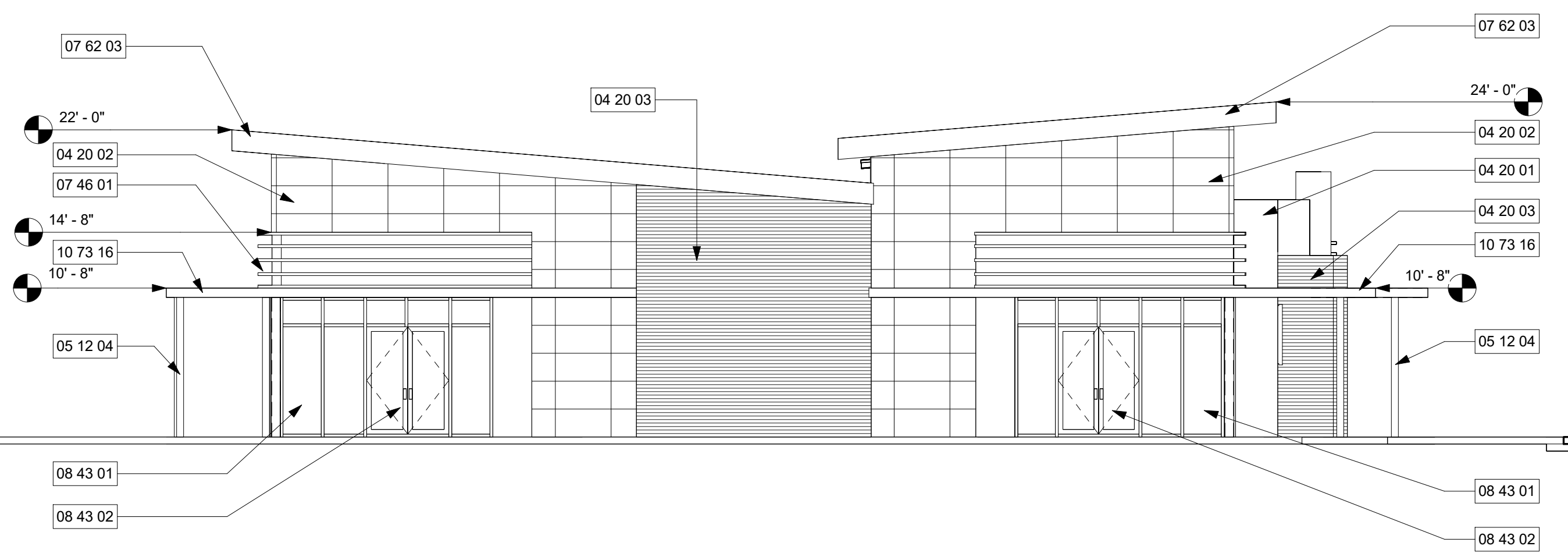
2 A3.01 EXTERIOR ELEVATION - NORTH-BW 1/8" = 1'-0"
