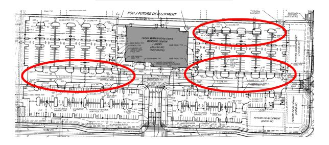
Proposed Site Plan Modification replacing pavers with painted ladder crosswalks
