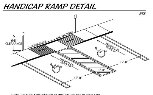
NOTE: IN THIS APPLICATION RAMPS CAN BE SEPARATED AND SIDEWALK CAN BE FLUSH ACROSS ALL HC SPACES NOTE: HCR#3-MOD MEANS ONLY 1 RAMP BUILT TO REQUIRED SIDE OF SIDEWALK. OR RAMPS SEP. TO ENDS OF HC SPACES NOTE: REFER TO ENGINEERING PLANS REGARDING PARKING SPACE STRIPING SINGLE VERSUS DOUBLE
