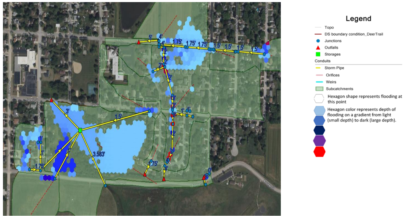
Figure 1. Existing flooding conditions in MRR6.6 during the 100-Year storm event.
