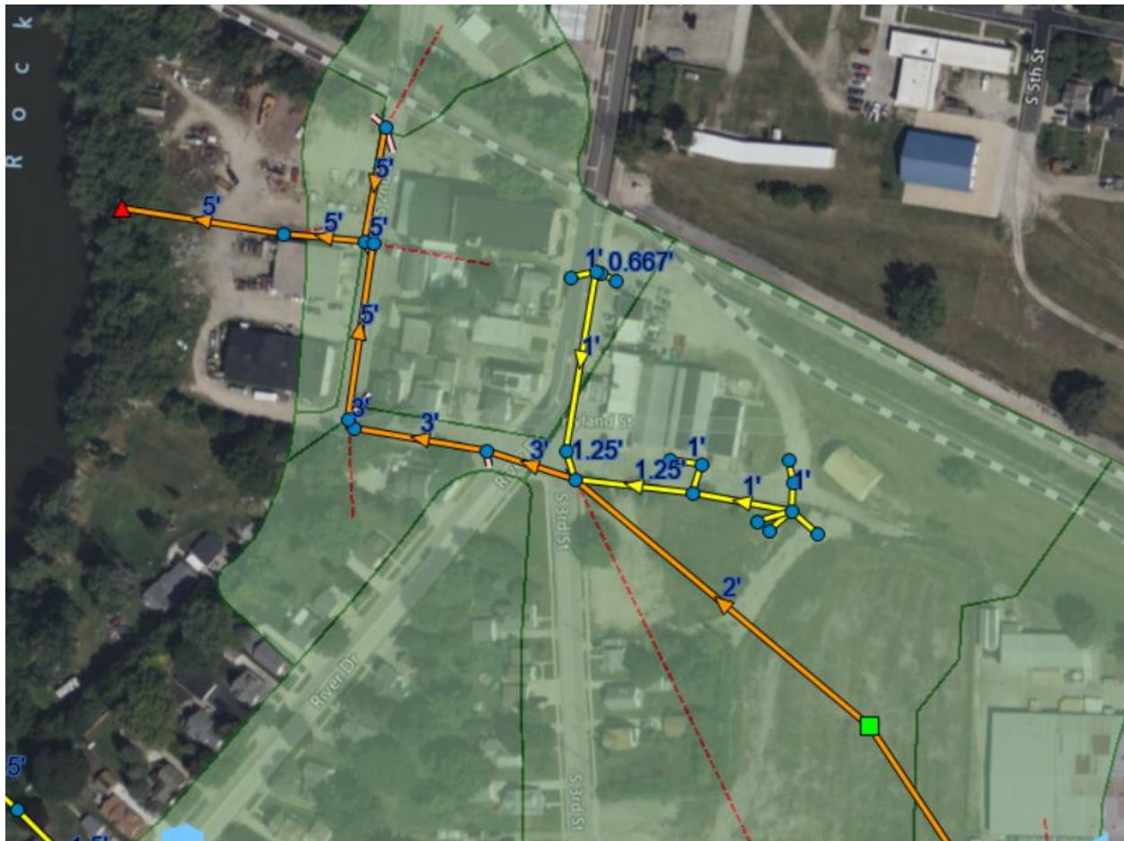
Figure 2. Flooding conditions after implementation of recommendations during the 100-year event at the intersection. Locations of proposed pipe upsizing are shown in orange. The proposed storm water facility is shown in light green. Approximately 2,300 lineal feet of 15-inch to 60-inch storm sewer will be provided as part of the proposed upsizing.
