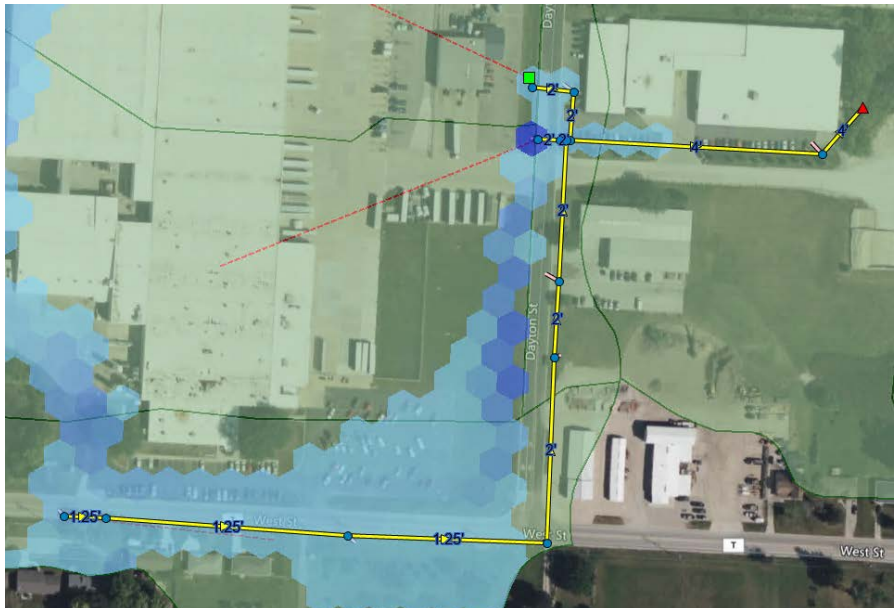
Figure 2. Flooding conditions after implementation of recommendations during the 100-year storm event along Dayton Street. The proposed storm water storage at WisPAK is shown in light green. The increase of flooding along West St. (CTH T) is the result of the pipes less than 18-inches included in the proposed conditions, however this flooding depth of 3.5 inches is not anticipated to be a concern during the 100-year event. The flooding along West St. is 0.3 feet within the street. The flooding area of concern is further north on Dayton St. where the flooding crosses the road.
