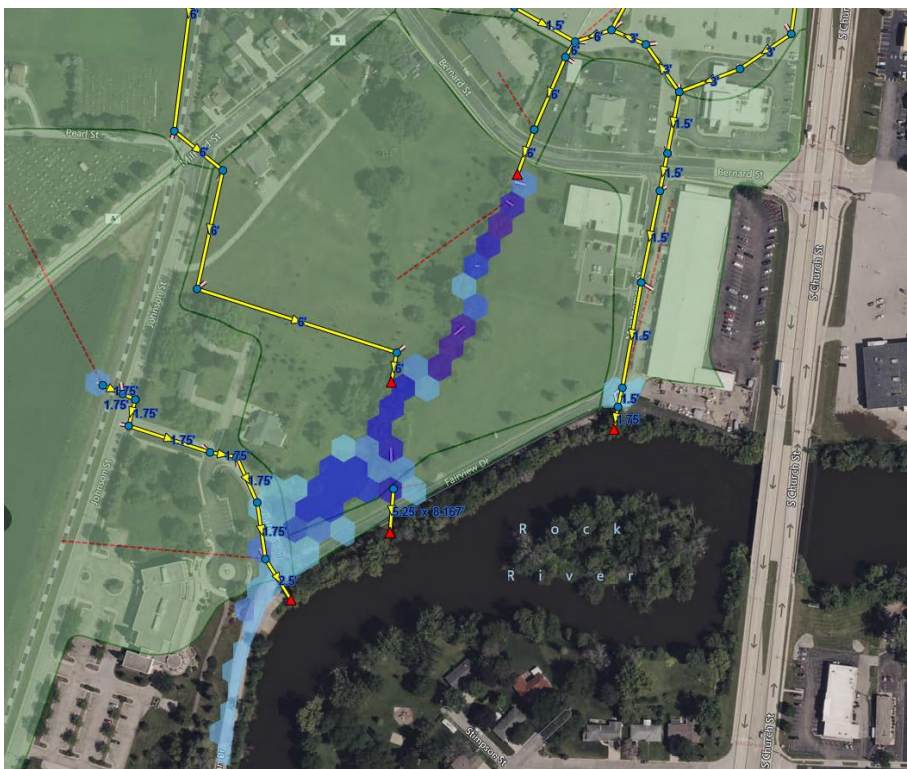
Figure 2. Flooding conditions after implementation of recommendations during the 100-year event at the intersection of Hoffman and Fairview Drives. Maximum flooding depth of 0.31 ft in this area of concern.
