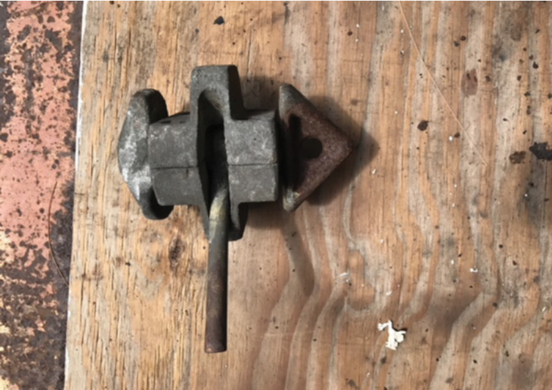
(2) There are several types of locking devices to secure the containers vertically and horizontally (Photo by Dave Dorsette.)
