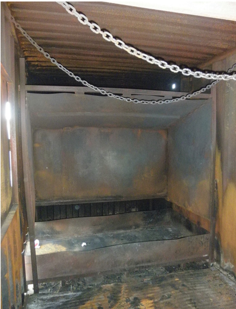
(11) A hearth to protect the container roof and walls; the drawer below is to collect staples, nails, and debris that can be slid out to the left and dumped. (Photo by author.)
