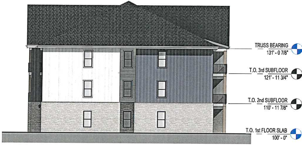
② BUILDING A - LEFT SIDE ELEVATION 1/8" = 1'-0"
