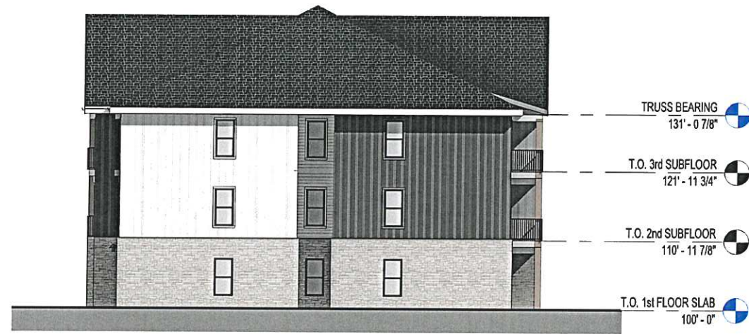
② BUILDING B - RIGHT SIDE ELEVATION 1/8" = 1'-0"
