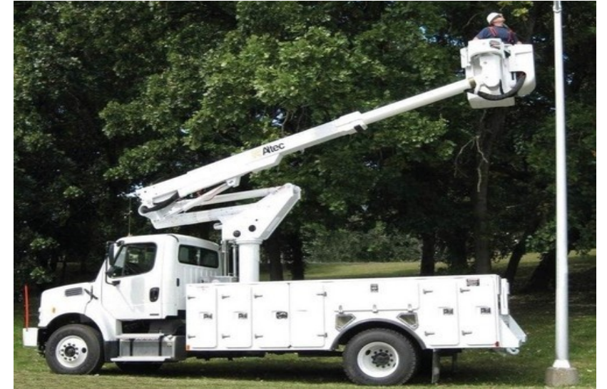
Aerial Cable Placement (Bucket Truck)
