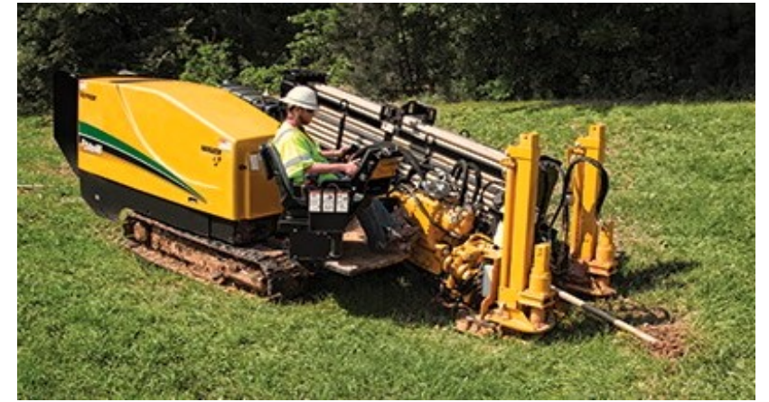
Buried Cable Placement (Directional Bore)
