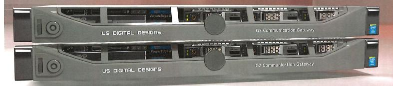
The G2 Communications Gateway is the link between the CAD system at the dispatch center and the G2 ATX Station Controller hosted at each fire station.
