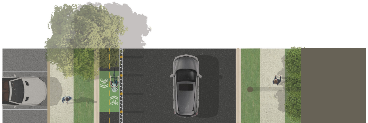
Figure 4.3 Cross section and plan view study of two-way protected bike lane on Market St.
