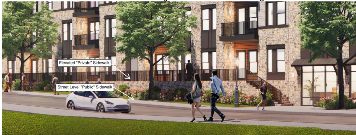
View of Section B Showing “Double Sidewalk” Configuration
