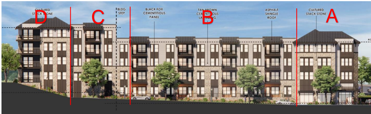
Profile Illustrating the “Stepping” of the Apartment Building
