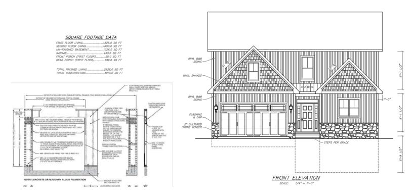
The image above shows the proposed elevations for the home, and includes square footage data for each floor, and all accessory structures. The first and second floors of the home are 2,926 square feet combined, the unfinished basement is 1,326 square feet, the garage is 440 square feet, and both front and rear porches are 222 square feet combined.
