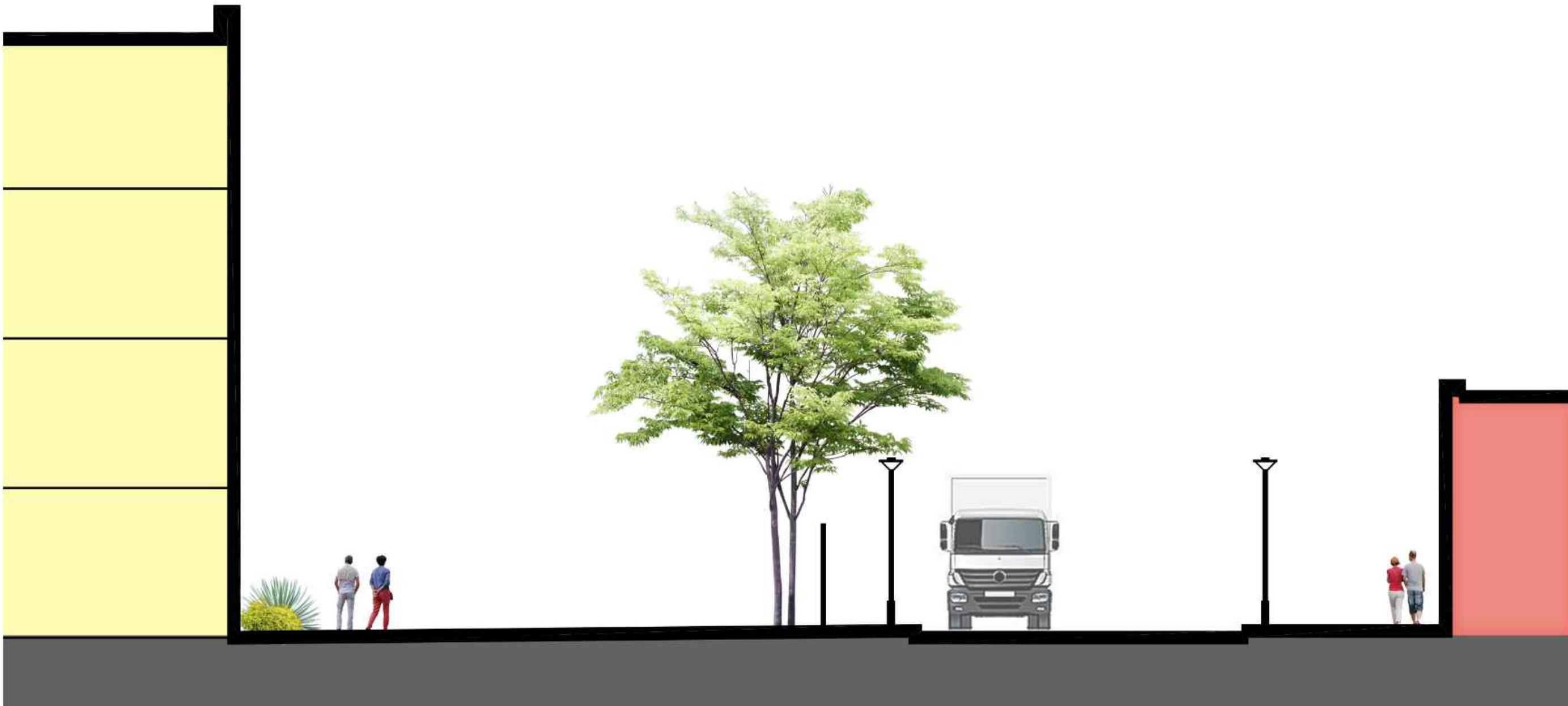
TYPICAL SECTION THROUGH ALLEY SCALE 1/8"=1'-0" GREEN BUFFER (VARIES) BETWEEN RESIDENTIAL AND ALLEY ALLEY SIDEWALK / RETAIL LOADING + TRASH ZONE ( VARIES)
