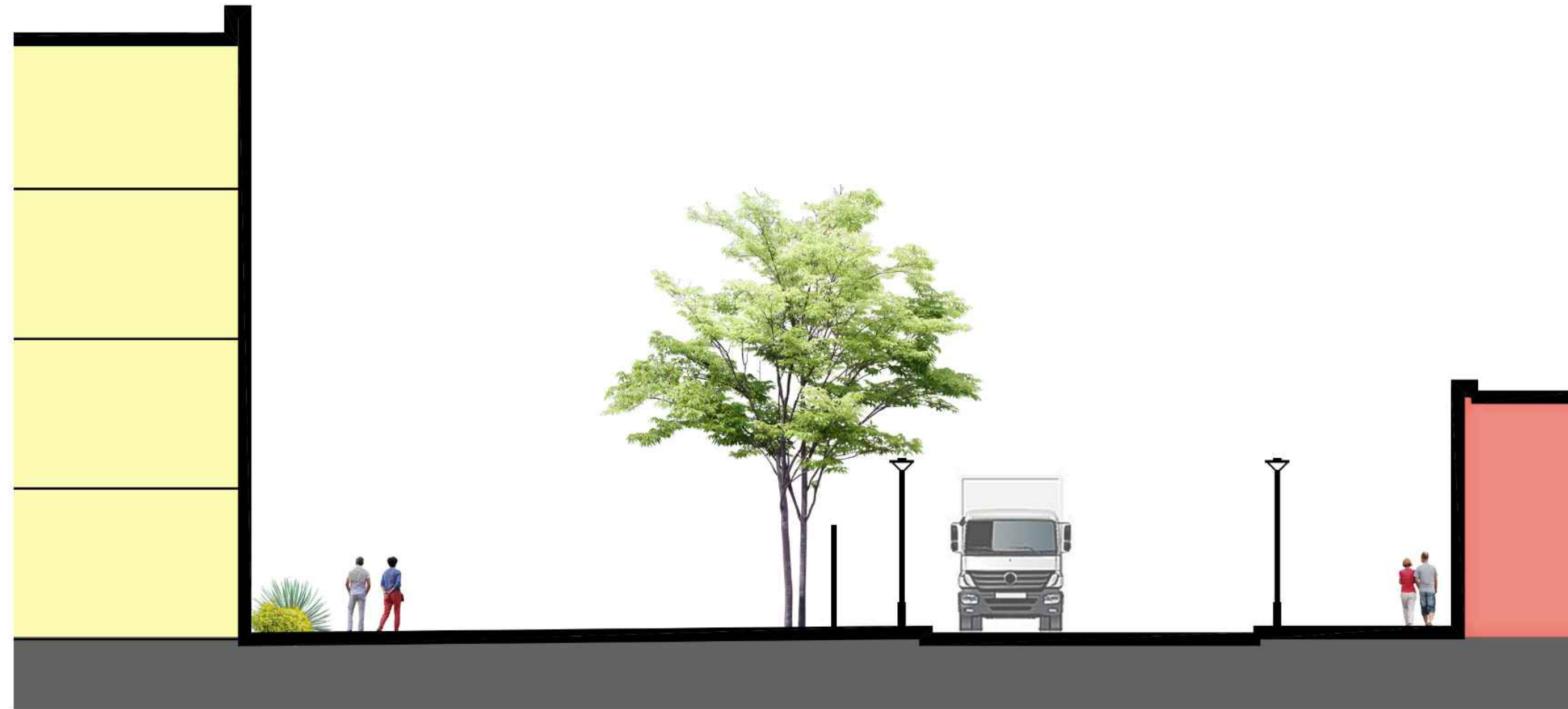
GREEN BUFFER (VARIES) BETWEEN RESIDENTIAL AND ALLEY ALLEY SIDEWALK / RETAIL LOADING + TRASH ZONE (VARIES) TYPICAL SECTION THROUGH ALLEY
