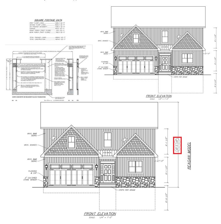
The images above show the proposed elevations for the home, and include square footage data for each floor, and all accessory structures. The first and second floors of the home are 2,926
