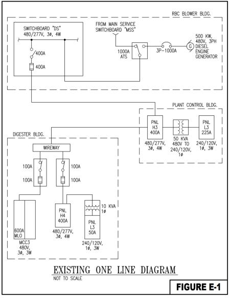
Figure 3: Existing Electrical One-Line Diagram
