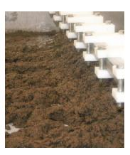
**2** Roto-Kone® Elements -Roto-Kone elements lift and decelerate incoming sludge creating a head which turns the sludge to enhance separation. Roto-Kone stations are placed in several locations along the entire length of the belt. The elements rotate, reducing rag hang-up, and self adjust to maintain contact with the belt. They can be lifted to precisely control final cake solids.
