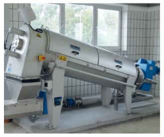
Stationary mounted screw press for 140 kgDS/h
