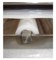
Belt Support/Wiper Bars - The dewatering belt is supported on abrasion-resistant, replaceable polyethylene wipers to enhance dewatering by constantly breaking the liquid surface tension. Wipers can be rotated providing multiple wear surfaces.
