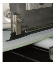
4 Side Seals - Replaceable rubber side seals prevent sludge from spilling off the sides of the moving drainage belt. A clamp is used to hold these seals in place for easy removal and installation.
