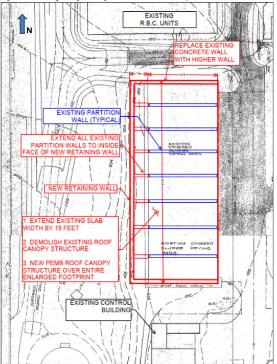
Figure 5 : Existing Sludge Storage Area Site Plan and Proposed Modifications
