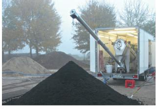
Contract dewatering with a trailer-mounted HUBER Screw Press Q-PRESS<sup>®</sup>
