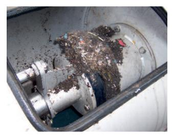
Discharge of the separated dewatered material
