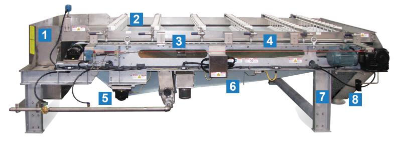
**5** Bearings - All bearings are a split pillow block, double-row spherical roller design. They lie outboard of the process stream, are regreasable, and are nylon coated. For our standard two meter machine the minimum L-10 life is equivalent to over 135 years of continuous service.
