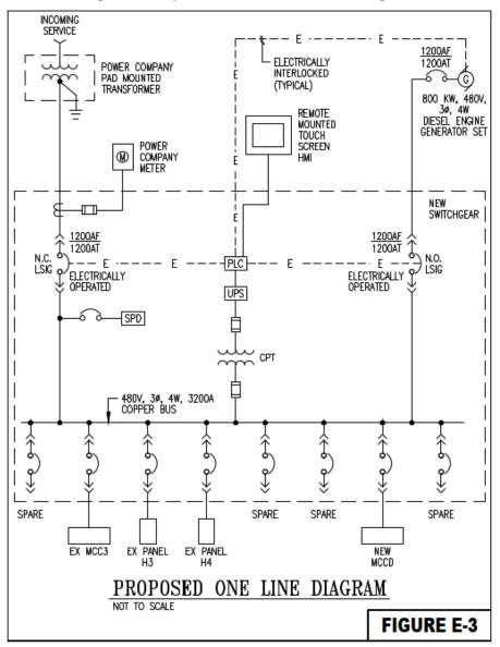
Figure 8: Proposed Electrical One-Line Diagram.
