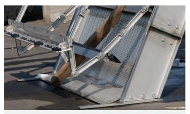
Factory demonstration of 4"x4" entering screen at bottom of channel.
