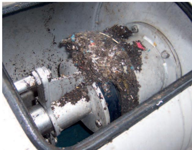
*Discharge of the separated dewatered material*
