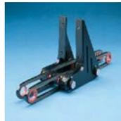
**Envirex® ENV715 Chain:** Manufactured out of Series 400 stainless steel with hardened pins and bushings, ENV715 collector chain provides excellent strength and corrosion resistance. This chain is suitable for applications with elevated grit levels or sludge loads where a stronger, more robust chain is required. It is especially suited for plants using stacked (double deck) collectors where the collectors can't be visually inspected or easily accessed.
