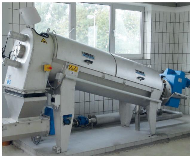
*Stationary mounted screw press for 140 kgDS/h*
