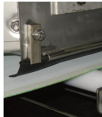
**1 Feed Section** - Polymer is injected through a multiport ring and mixed with the sludge via a non-clog variable orifice mixer in the feed line prior to entering the flocculation tank. Coagulated solids form in the flocculation tank and overflow onto the dewatering belt in a smooth, gentle stream, minimizing floc shear.
