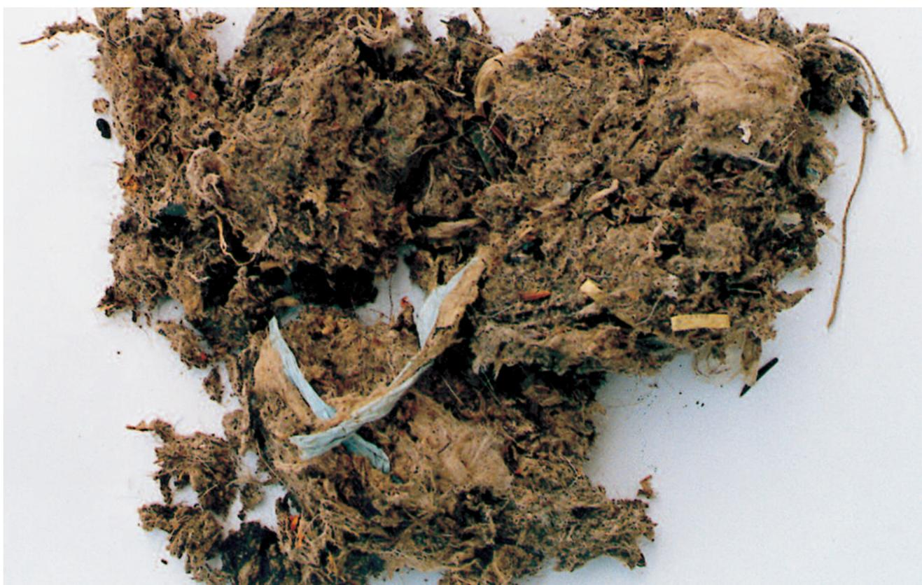
*Separated material: paper, wood, plastic, foils, rubber, textiles, etc.*
