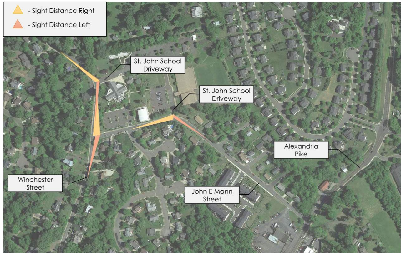
Figure 14. Sight Distance near St. John's School
