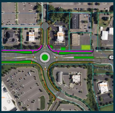
General Concept is to install a roundabout to keep circulation moving with the other roundabouts and improve safety. Final Design to be determined.
