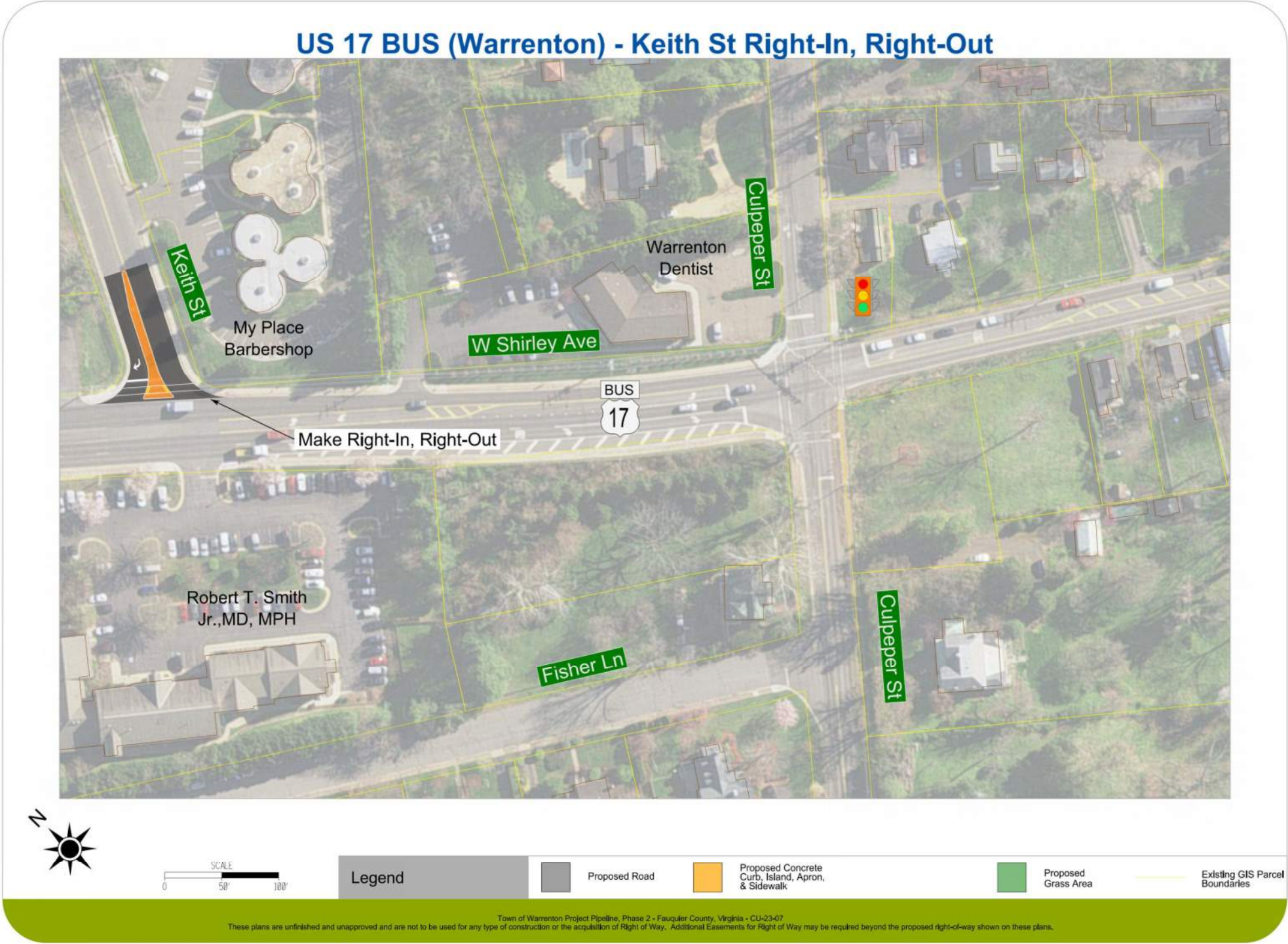
Figure 2-5: Keith Street Right-In, Right-Out Layout
