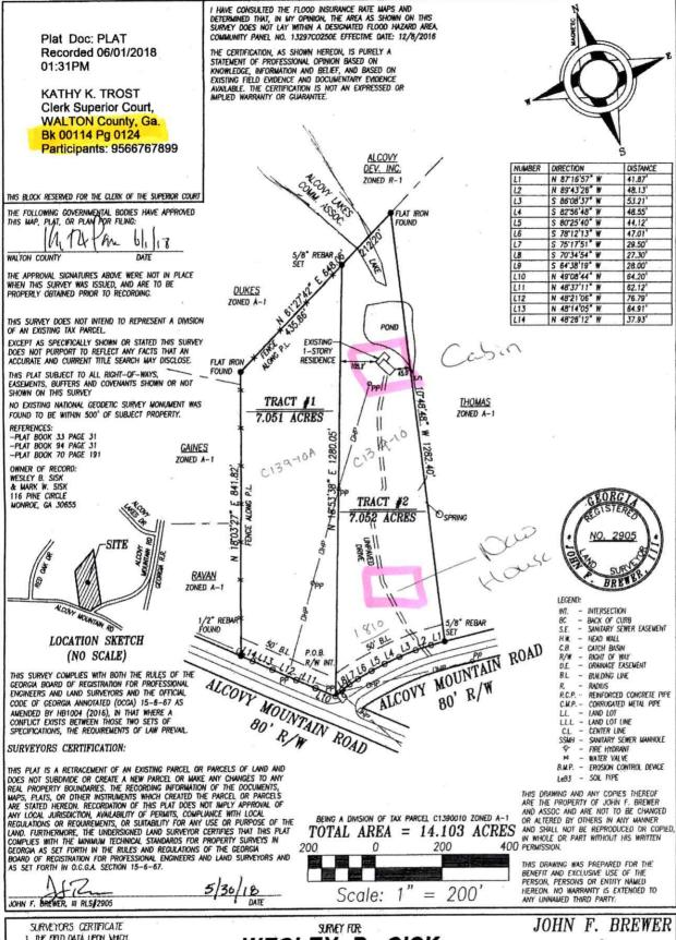
1. THE FEED DATA UPON WHICH THIS PLAT IS BASED HAS A CLOSURE PRECISION OF ONE FOOT IN 38,574 FIET AND AN ANGULAR ERROR OF 2 SECONDS PER ANGLE POINT
