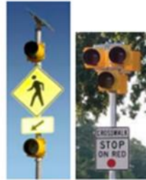
Standard and Hawk Mid-block Pedestrian Crossings
