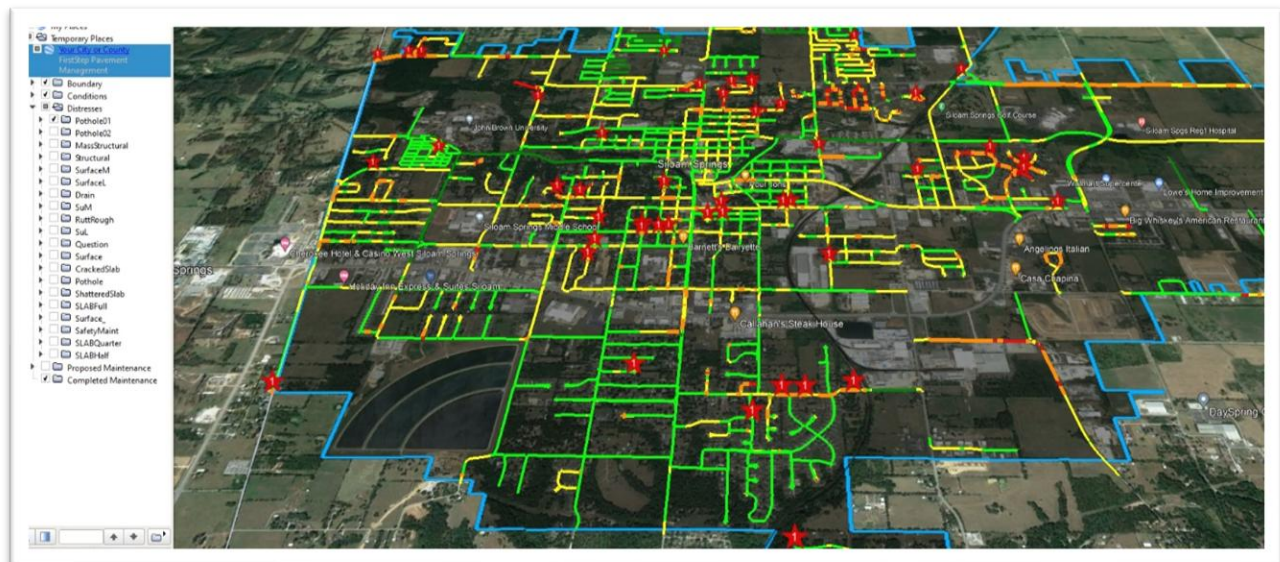
Figure 1 – Dynamic Condition Map with Road Condition and Distress Toggle Buttons
